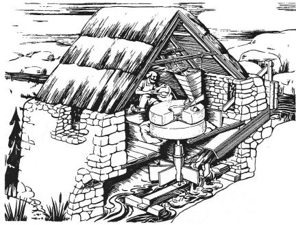
FIGURE 1-5. Horizontal watermill. These rather inefficient mills did not utilize gearing and usually required a relatively small volume of water with a modestly high fall. Their chief asset was low first cost.
